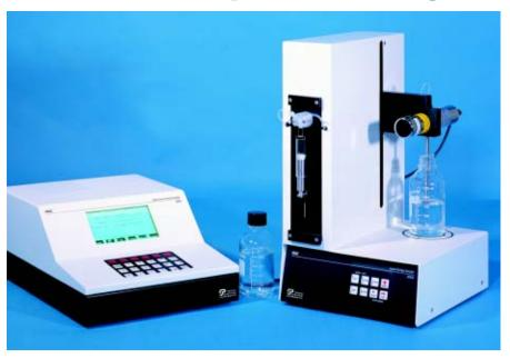
The HIAC Model 8103 System is a versatile system for use in parenteral particle counting of SVI and LVI for USP 24 <788>, JP and EP, and precision cleaning applications. The 8103 System is easy to use, reduces sampling costs, and uses proven particle counting technology. This system is ideal for qualification of cleanliness levels using water, solvents, and chemicals. The 8103 System works with the HRLD and MicroCount sensors to measure particles from 0.1 to 400 microns.
