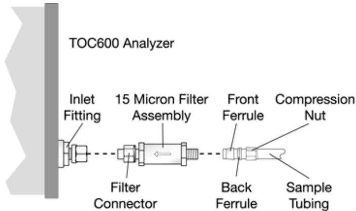
Fig 2-19 : TOC600 Analyzer
