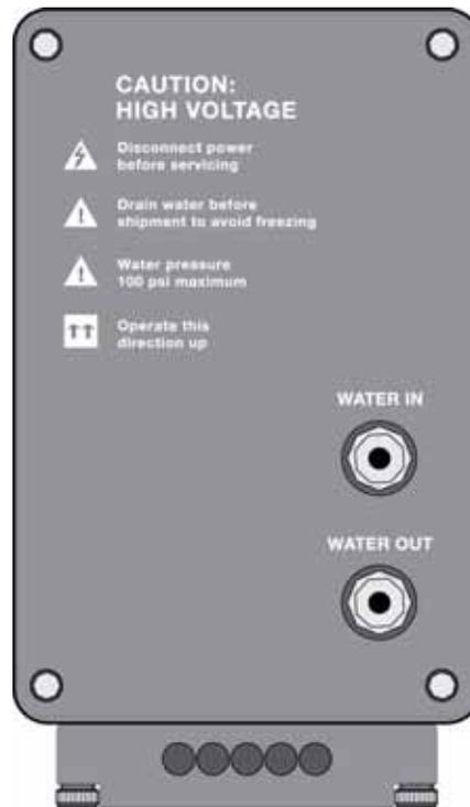
Fig 2-20 : TOC600 Analyzer Water I/O Connections
