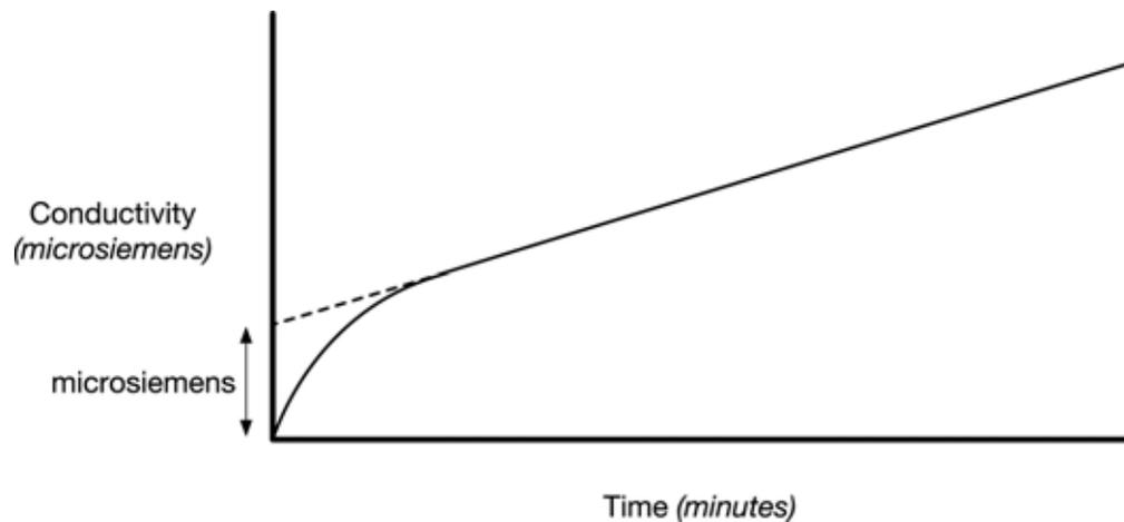
Fig 5-14 : P2-Type Oxidation Curve
