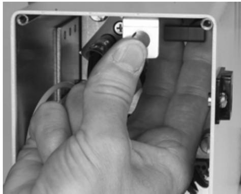
*Fig 13-8 : Pulling the UV Lamp Connector Plug*
