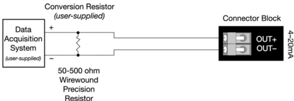
Fig 9-2 : Voltage Output Wiring
