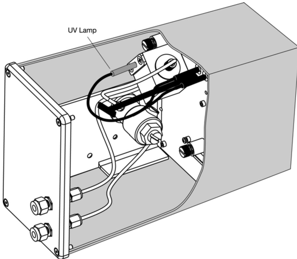
Fig 13-6 : TOC600 Analyzer UV Lamp Replacement Diagram
