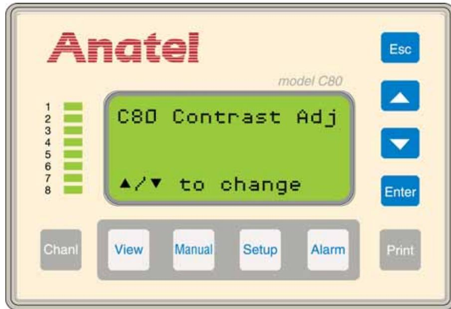
Fig 4-4 : C80 Contrast Adjustment Screen
