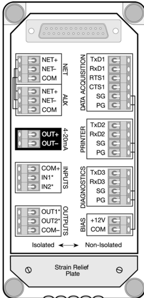
Fig 2-22 : Connector Block
