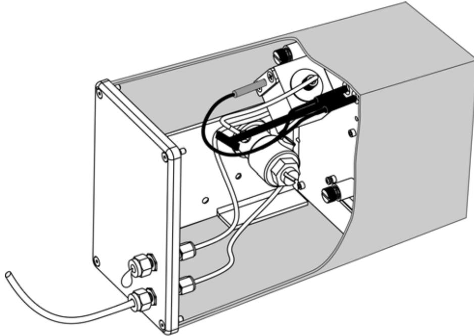
Fig 14-2 : Purging the TOC600 Measurement Cell
