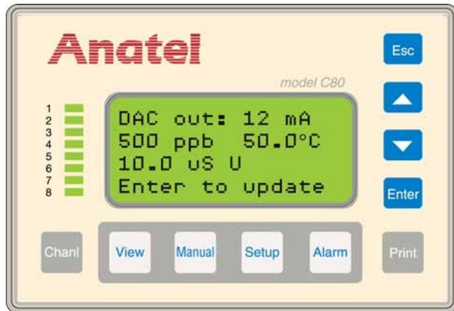
Fig 14-9 : DAC Output Test Screen
