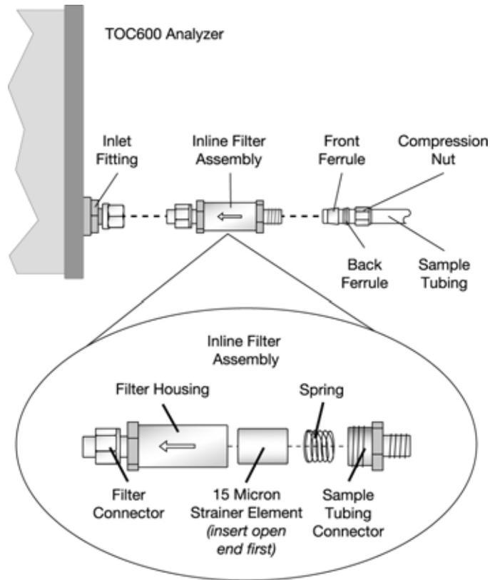
Fig 13-14 : In-line Filter Assembly
