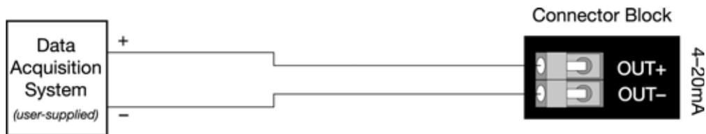
Fig 9-1 : Current Output Wiring
