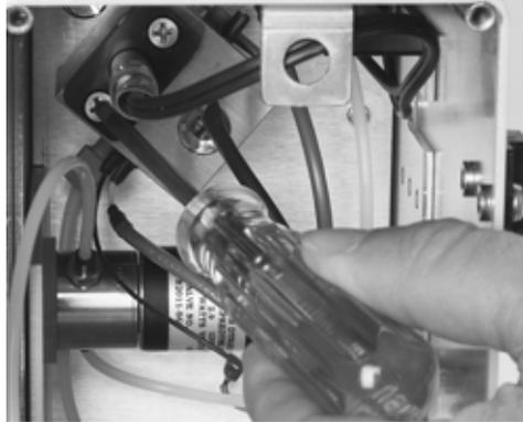
*Fig 13-7 : Loosening the UV Lamp Bracket*
